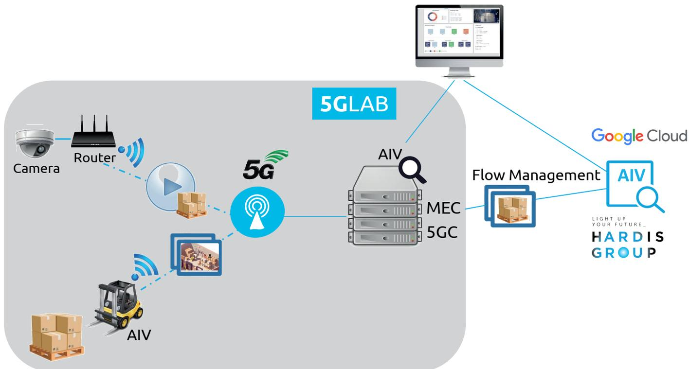
In the next step of the Demonstrator, dynamic network slicing features will be applied. Network KPIs will be continuously analyzed to dynamically create a new slice for the AIV and guarantee the latency performances when SLA required by the AIVs are not fulfilled anymore.
