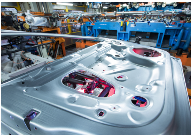
Figure 5: Quality inspection of metal sheets at Audi’s Ingolstadt press shop
