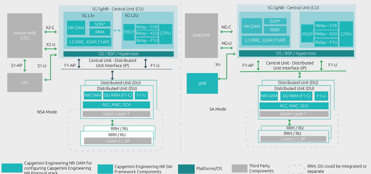
Figure 2: Note: Above view is a logical module view of Capgemini Engineering NR Software Components vis-à-vis gNB Solution.
